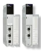
The QUCM is a programmable communication module for the Quantum PLC with two serial ports and an optional Ethernet port. The QUCM runs compiled structured text language programs that feature a real-time clock, a TCP/IP stack, and a large number of internal registers. Niobrara offers programming services to provide drivers for custom applications with many free to download from our Web site at www.niobrara.com. The QUCM is fully Unity Pro compatible.
