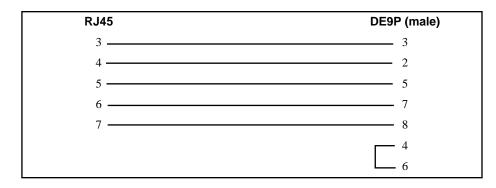
The Niobrara MM3 cable may be used for providing the CUCM with a 9-pin port that acts like a personal computer's serial port.
