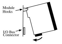
Figure 1-2 Mounting the CUCM on the Backplane
