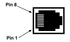
Figure 9-2 Ports 1 and 2 RJ45
