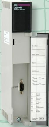
**“When the QSPXM serves as the host for the Seriplex network, no clock module is needed...serves as the source of pull-up current...”**
