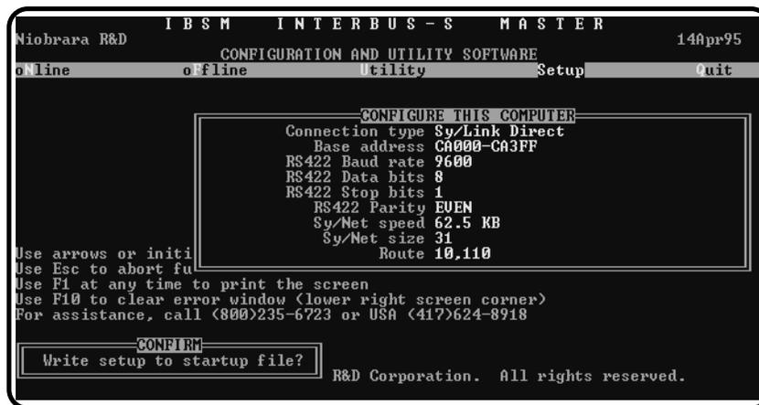
Figure 4-15 SY/LINK Setup Screen
