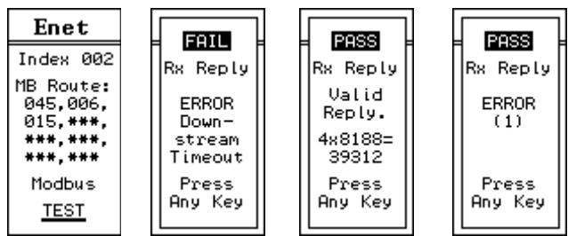
Figure 3.4: Modbus Route Edit TEST Screens
