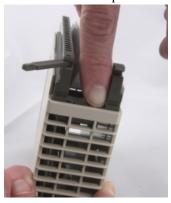
Now let the straight side of the cover lay down onto the side of the module.
