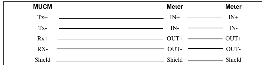
Figure 2-3 MUCM to 4-wire Modbus Slaves
