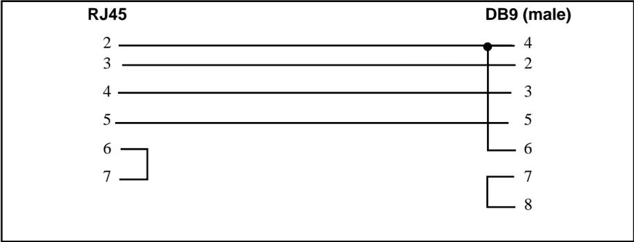
**Figure 2-1 QUCM-OE to Modicon RS-232 Port (9-pin) (MM2 Cable)**
