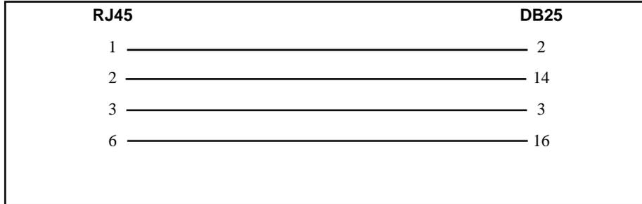
Figure 4-2 QUCM-OE RS-422 to Helm Loadgard Serial Interface
