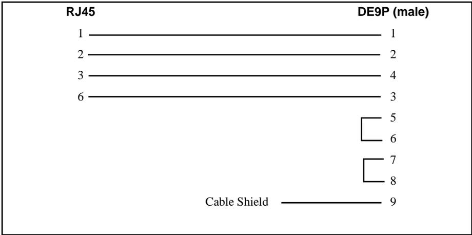
**Figure 2-2 RS-485 SY/MAX Port (9-pin) (MM7 Cable)**
