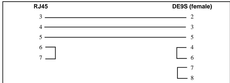
**Figure 2-4 QUCM-OE to RS-232 PC DCE Port (9-pin) (MM1 Cable)**
