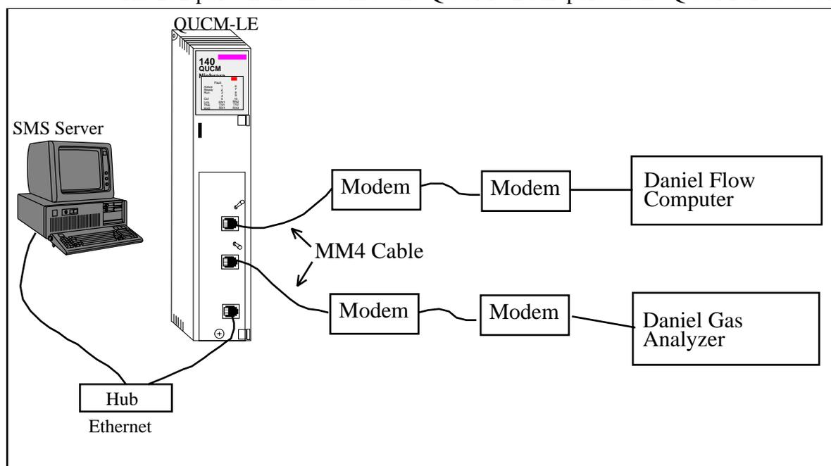
**Figure 4-1 Ethernet Network Example**
