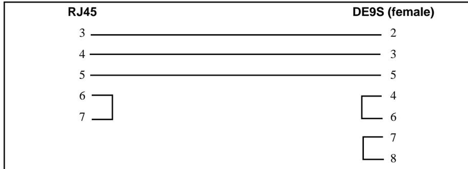
Figure 2-2 QUCM-SE to RS-232 PC DCE Port (9-pin) (MM1 Cable)
