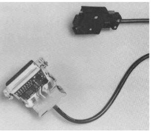
The SC50I can be used for communication between a personal computer and one Model 50 only. It cannot be used to communicate through the Model 50 network. However, it can of course be used to program individual Model 50's which will be interconnected in a network during operation. To connect a personal computer to a network of Model 50's, use the Square D NLU and Niobrara's **SC902** cable.
