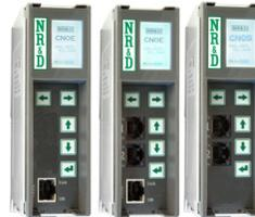
The CNOE/CNOS are communications modules for the TSX Compact PLC. They are available with Ethernet only, serial only, or Ethernet with serial. The Ethernet is 10/100BaseT and supports Modbus/TCP. The serial ports are switchable RS-232/485 supporting Modbus and 17 other protocols. Concept and ProWORX programming is supported, along with MSTRs and I/O Scanning.
