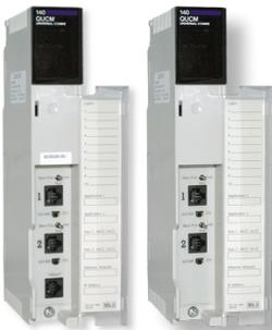
The QUCM is a programmable communication module for the Quantum PLC with two serial ports and an optional Ethernet port. The QUCM runs compiled structured text language programs that feature a real-time clock, a TCP/IP stack, and a large number of internal registers. Niobrara offers programming services to provide drivers for custom applications with many free to download from our Web site at [www.niobrara.com](http://www.niobrara.com). The QUCM is fully Unity Pro compatible.
