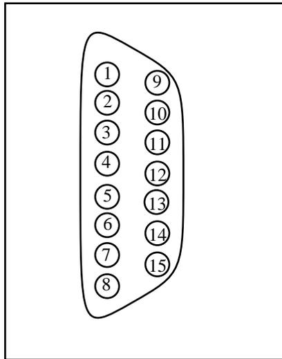
**Figure 5-1 AUI Connector Pinout**
