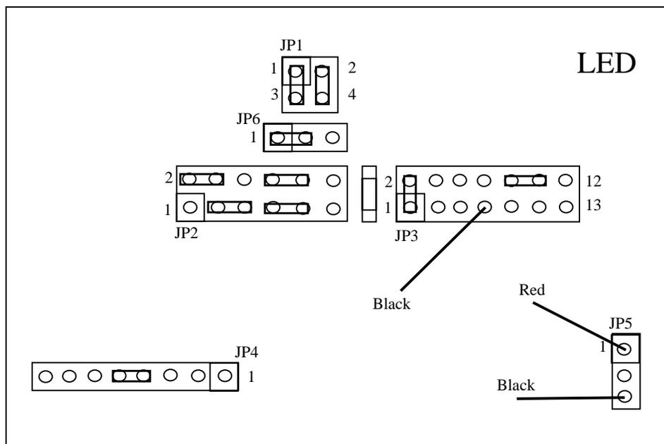
**Figure B-1 Jumper Setting for Upgrading NET I/O to STU firmware.**
